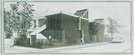
Two wedge-shaped, monopitch roofs bring in "north light" — daylight, not direct sunlight. The inverted plan, with family living space on the top floor and the children's bedrooms below — benefits from this. Photovoltaic panels power lights and triple-A-rated appliances; solar panels provide hot water. All are angled 40 degrees south for best performance.
